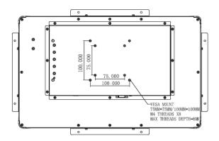
Drawing for illustration only. The VESA pattern on TMO101 is 75mm x 75mm.
