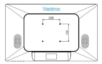
Drawing for illustration only. The VESA pattern on TMC156 is 75mm x 75mm. Screw specifications:
