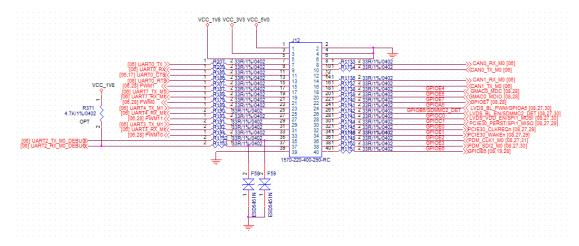
The CAN buses on the GPIO header operate at 1.8V levels without on-board transceivers. It is recommended to install external CAN transceivers and a  $120\Omega$  termination resistor to each bus before connecting to a network.
