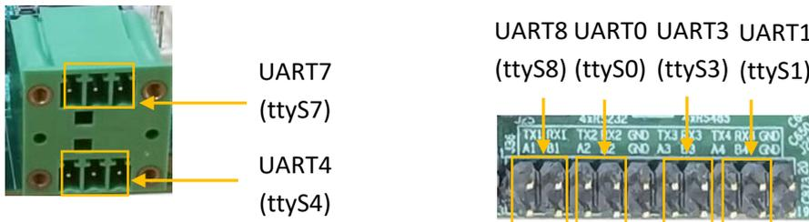
*You can use a proper USB-to-serial adapter to connect one serial port and the host computer first (TX-RX, RX-TX, GND-GND for RS232 wiring, A-A, B-B, GND-GND for RS485 wiring), then use a serial communication program to check if the serial port functions properly.*
