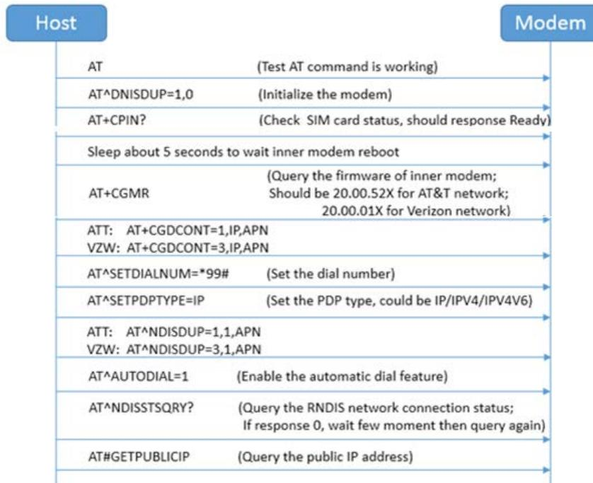
Below is a list of the AT commands that could be used for querying the status of the cellular card (“modem” equals the cellular card).
