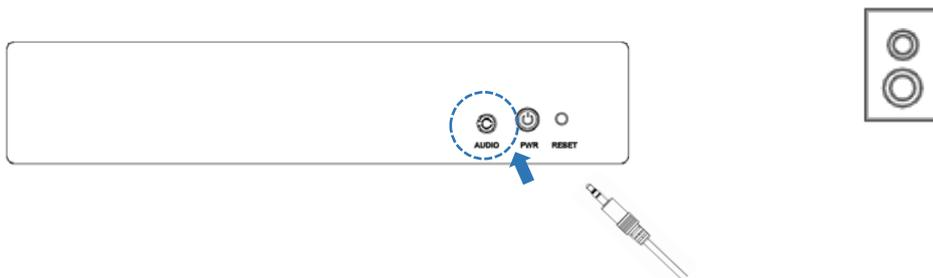
7. Connect the power cord to the DC jack of the device and plug the 12V/24V power adapter into a power receptacle to power on the device;
