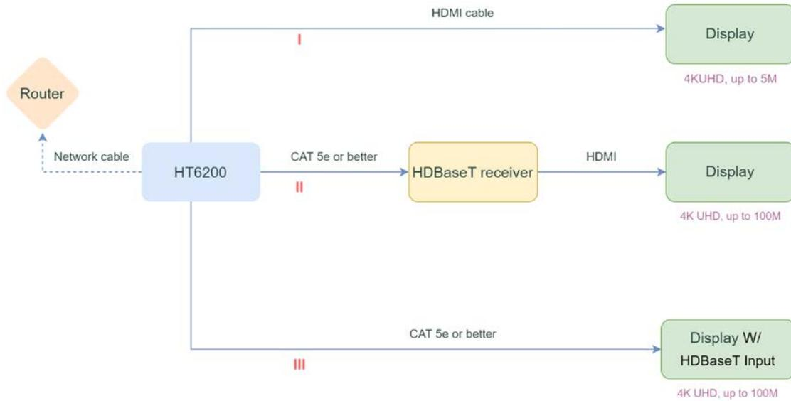
Scenario 1: Use an HDMI cable to connect HT6200 to a display for 4K UHD output at a maximum distance of 5 meters.
