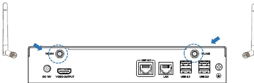
▶ *If only one Wi-Fi antenna is shipped, install it to the WLAN1 connector for better signal strength.*
